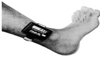
FIG. 3. — PAM-RL records leg movements continuously for up to 72h differentiating between standing and lying position using an integrated position sensor. Somnomedics®.
